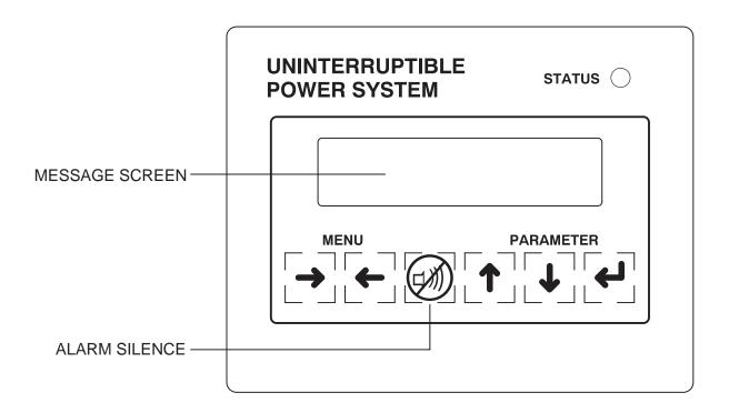
Figure 3–1. Digital Monitoring Panel
